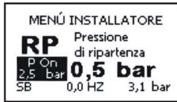
Figure 13: Setting the restart pressure
