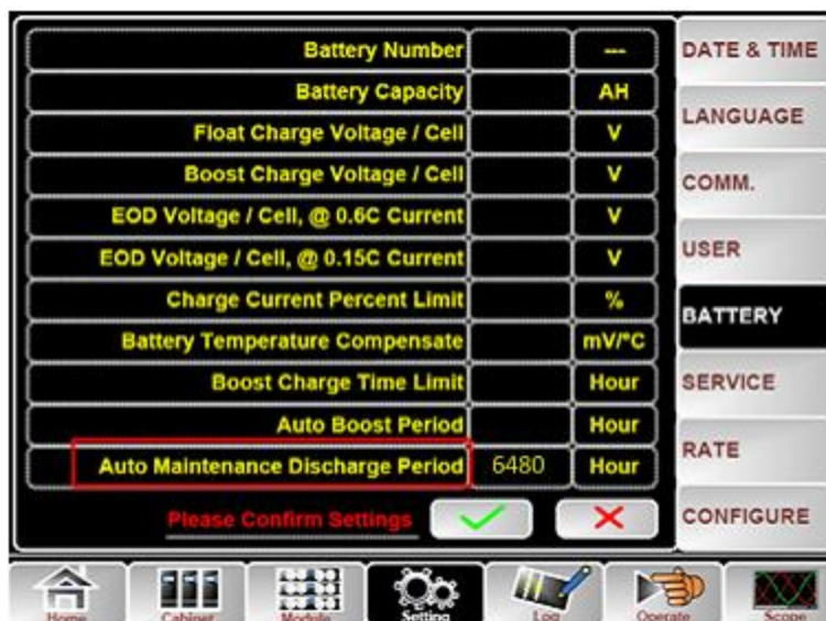
Fig.4-5 Setting period for battery auto discharge
