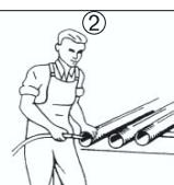
Clean out pipe before use. Pipe scale and dirt are often the cause of leaking valves.
