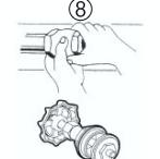
When cramped for room, remove the bonnet to ease installation.
