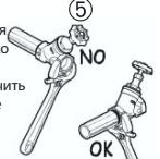
For assembly purposes, use a spanner, not a pipe wrench, by applying necessary working torque only on the valve end nearest the pipe. This helps get a firmer grip and avoid potential damages to the valve body.
