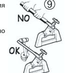
When mounting the bonnet on the valve body it is advisable to fasten it smoothly to prevent the sealing packing placed between these two small parts from undergoing excessive stress.
