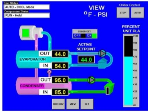
Figure 3, MicroTech II Controller Home Screen
