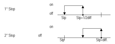
• Three steps Control: The first relay is enabled when reached the value of the Setpoint + 1/3 of the differential. The second step is enabled when reached the value of Setpoint + 2/3 of the differential. The third step is enabled when reached the value of Setpoint + the differential. Steps will be disabled as per the following schematic:
