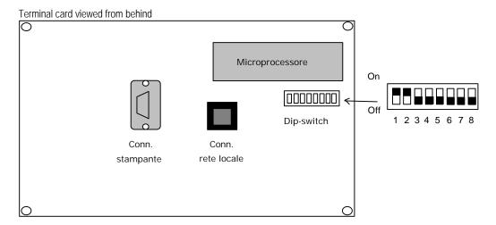
The address of the terminals is set up through the dipswitch bench found on the back . The address is selectable in the 1-16 range by utilising the 1-5 dipswitch. The address value is obtained via the following table (see also previous paragraph):
