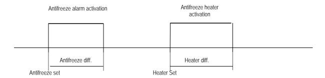
The antifreeze regulation is always energized also when the machine is OFF, both summer working and winter working.
