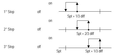
N.B: the number of steps controlling the cooling tower is selectable by keypad under "User" password.
