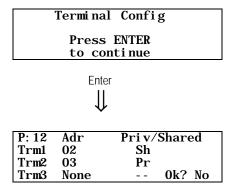
• In this mask the Enter button moves the cursor from one field to another whereas the arrow-buttons change the current value of the field. The P:12 symbol in this case indicates that the I/O address-12 card has been selected.
