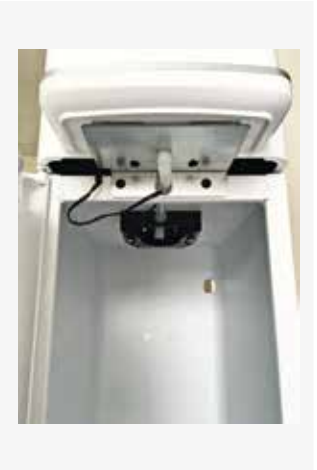
Fig. 9: Interior of the AQA drink Pro 20 cabinet without wastewater tank in place
