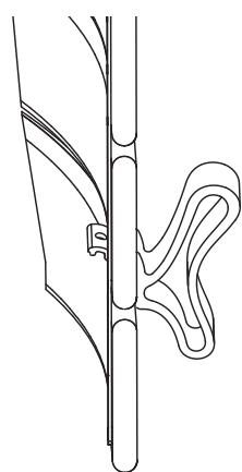
Fit the bolt and slide it in up to the stop.
