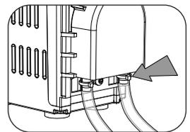
Situate the red sensor in the 'air on' side and the blue sensor in the 'air off' side of the evaporating coil.
