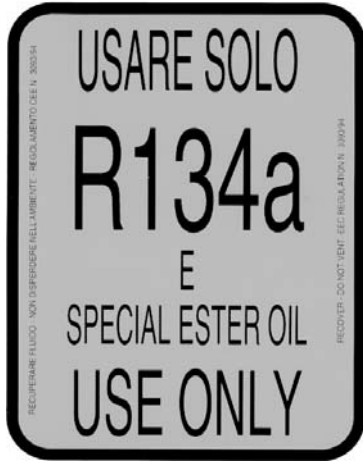
Identification of the refrigerant - External door
