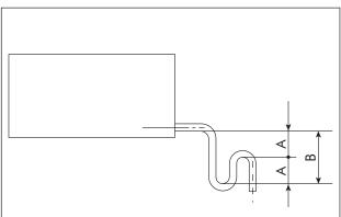
The height A must be equal to **2 times** the value of the negative pressure present in the condensate reception zone (example: negative pressure = 40 mm, height A = 80 mm, height B = 160 mm).
