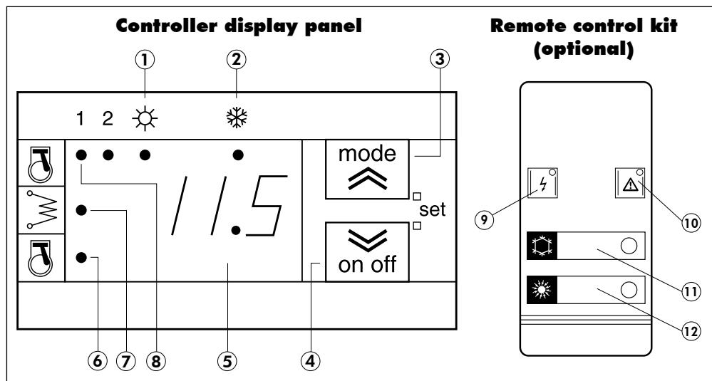
The controller provides information on status of operation, configuration and alarms through a display and LEDs on the front panel.
