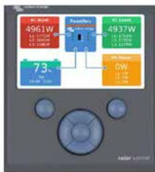
Color Control GX, showing a PV application
