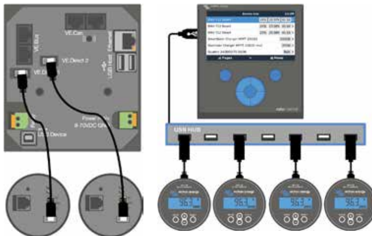
A maximum of four BMVs can be connected directly to a Color Control GX. Even more BMVs can be connected to a USB Hub for central monitoring.
