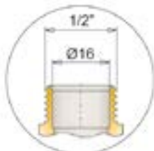
ART. 1668 (1/2") per tubi multistrato for multilayer pipe Ø14x2,0 Ø16x2,0 Ø18x2,0 Ø20x2,0
