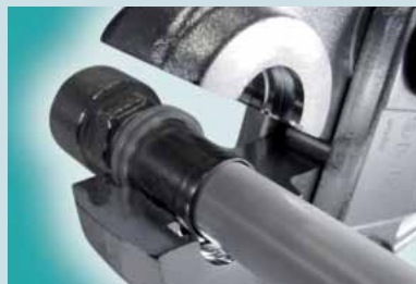
Exact position of the press-fitting (profile TH plier).
