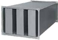
The silencer housing is made of galvanized steel. Sound-absorbing plates consist of non-combustible basalt fiber mineral wool covered with fiberglass to prevent blowing particles out.
