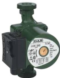
Designed for moving water and non-freezing mixtures with a temperature from -10 °C to +110 °C. Maximum possible operation pressure of the heat medium is 1 MPa. Motor shaft should be located strictly horizontally while mounting.
