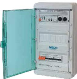
Soft start and protection of three-phase fans from 0.37 to 45 kW, not equipped with thermal contacts or thermistors (built-in UPP device). Overload protection with current-limiting circuit breakers.
