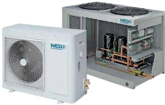
Condensing units are designed for the preparation of refrigerant transferred to the heat exchanger of the inner unit or to the section of direct evaporation in the air conditioning system. Non-reversing single-circuit (NSK and ND-SPL) and twin-circuit compressor-condensing (NSK) with axial fans and rotary/scroll compressors in 27 standard sizes with a capacity from 2 to 255 kW. Outdoor design of the units. Used refrigerant: R410A.
