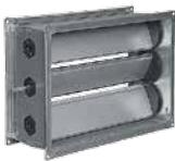
The damper body is made of galvanized steel, and the air blades are made of aluminum. The rubber seals on the edges of the blades. A pivoting square rod with a side of 10 mm ensures reliable locking of the damper actuator.
