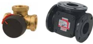
Used as mixing or separating valves for heat exchangers installed in ventilation and air conditioning systems. Rotary type valves with threaded (VRG131 series) or flanged (3F series) connection.
