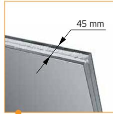
The 45 mm thick sandwich panels are made of two galvanized steel with lightweight polyurethane foam filler between them. Effective reduction of noise and heat loss as well as improved strength and rigidity of the structure of sections are provided
