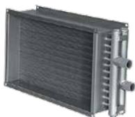
WH heaters are available in a double row and triple row design. The body is made of galvanized steel. The surface of the heat exchanger is made of aluminum fins and copper pipes passing through them in a checkerboard pattern. Designed for operation at a maximum working pressure of 1.5 MPa and a maximum working temperature of the heat carrier of 170°C.
