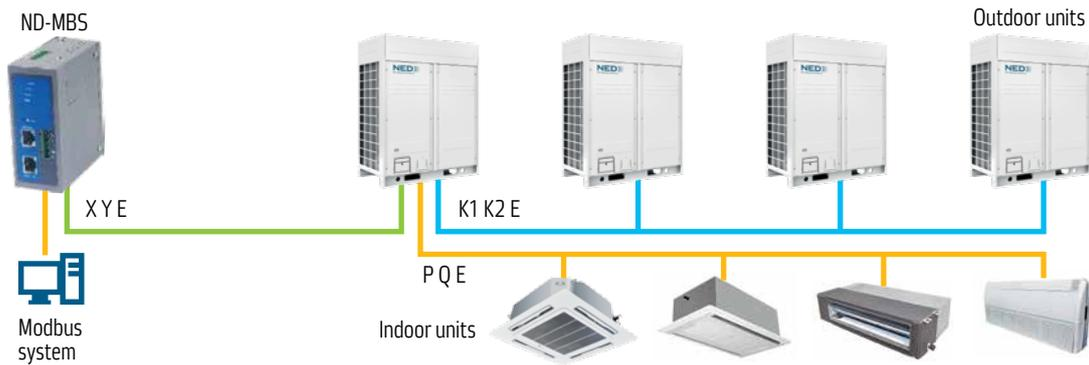
BacNet protocol — ND-BNT gateway. Supports the connection of MAX 128 indoor units or 4 outdoor units.
