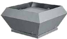
The fan housing and impeller are made of galvanized steel. The backward curved impeller is used. Single-phase and three-phase asynchronous electric motors are protected from overheating with the help of embedded heat contacts with remote circuit terminals. Operating resource is more than 50,000 hours. The fans are mounted horizontally on flat-deck or slanting roofs.
