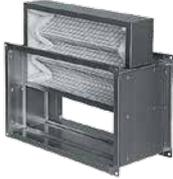
Body of filter and inserts are made of galvanized steel. The removable cover has special mounts for easy replacement and removal of the filter insert. FRC cassette filters are designed to work with DFC filter inserts. DFC filter inserts are not included. The filter element of the cleaning class EU3 is a non-woven cloth made of synthetic fibers, mounted on a galvanized steel mesh to protect against deformation by air flow.
