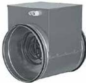
Housing and junction box are made of galvanized steel. Heating elements are made of stainless steel. Protection against overheating of the housing and air with two thermostats and a thermal contact circuit. The operating temperature range of the passing air is from -40°C to +40°C.
