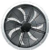
The fan housing and duct shell are made of galvanized steel. The crescent blades are manufactured by Ziehl-Abegg AG, Germany. Single-phase and three-phase asynchronous electric motors are protected from overheating with the help of embedded heat contacts with remote circuit terminals.
