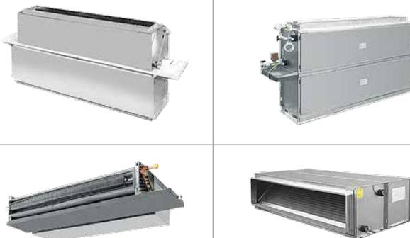
Low-pressure (up to 30 Pa) ducted fan coils are represented in six standard sizes with overall cooling capacity from 2.1 kW to 10.8 kW. Middle-pressure and high-pressure ducted fan coils are represented in eleven standard sizes with an overall cooling capacity from 4.2 kW to 42.8 kW.
