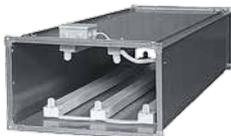
Air sanitising by means of ultraviolet bactericidal irradiation. Body is made of galvanized steel. The sections are equipped with low pressure mercury gas-discharge bactericidal lamps with a power of 36 W and 75 W and a voltage of 230 V.
