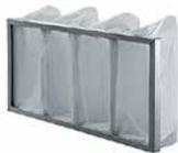
DFU filter inserts for FRU pocket filters. DFU filter inserts have a cleaning class of EU3. The filter element is a non-woven cloth made of synthetic fibers, mounted on a frame in the form of pockets.
