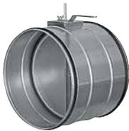
The body and the flap of the damper are made of galvanized steel. Hermetic rubber seal on the edge of the flap. A manual mechanism with an angle lock is included in the standard supply. A pivoting square rod with a side of 8 mm ensures reliable locking of the damper actuator.
