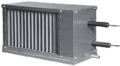
The heat exchanger has single- circuit three-row design. The casing is made of galvanized steel. The surface of the heat exchanger is made of aluminum fins and copper pipes passing through them. All coolers are equipped with a profile plastic droplet eliminator and a condensate tray with catch&drain manifold for collecting and draining condensate. Optional installation of a capillary thermostat to protect the cooler from frosting is available.
