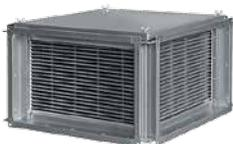
Efficiency of exhaust air thermal energy use reaches 70%. Body is made of galvanised steel. The heat exchange surface represents a package of 0.2 mm thick specially shaped aluminium plates. Complete set includes a pan and nozzle with a fastening nut for draining of condensate.
