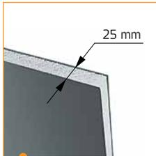
The 25 mm thick sandwich panels are made of two galvanized steel with lightweight polyurethane foam filler between them. Effective reduction of noise and heat loss as well as improved strength and rigidity of the structure of sections are provided
