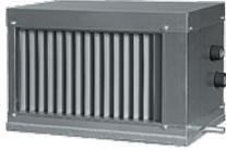
The heat exchanger has three-row design. The casing is made of galvanized steel. The surface of the heat exchanger is made of aluminum fins and copper pipes passing through them. All coolers are equipped with a profile plastic droplet eliminator and a condensate tray with catch&drain manifold for collecting and draining condensate. RW coolers are designed for operation at a maximum working pressure of a coolant of 1.5 MPa.
