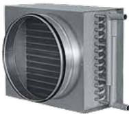
A double row design. The body are made of galvanized steel. The surface of the heat exchanger is made of aluminum fins and copper pipes passing through them in a checkerboard pattern. Designed for operation at a maximum working pressure of 1.5 MPa and a maximum working temperature of the heat carrier of 170°C.
