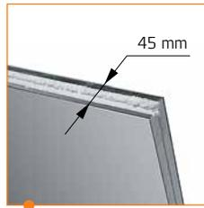
Sandwich panels with a thickness of 45 mm are two galvanized steel with lightweight polyurethane foam filler. Effective reduction of noise and heat loss, as well as increased strength and rigidity of the sections
