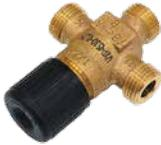
Used as mixing or separating valves for heat exchangers installed in small ventilation and air conditioning systems. External thread. Valve rod travel is 5.5 mm. Complete set does not include fittings.
