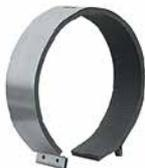
These clamps are intended for the simple and convenient installation of circular ventilation systems' components, as well as for the prevention of vibration transmission from the fan to the air duct. The clamps are made of galvanised steel with an insulating sealing layer. They are tightened with two bolts.
