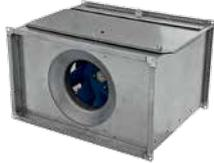
The fan housing is made of galvanised steel and has a removable service cover. Durable and light “free” impeller with backward bent blades made of polyamide reinforced with glass fibre is installed directly on the electric motor’s shaft. Three-phase asynchronous electric motors are protected from overheating with the help of embedded heat contacts with remote circuit terminals. Insulation category: IP 54.
