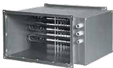
Housing and junction box are made of galvanized steel. Heating elements are made of stainless steel. Protection against overheating of the housing and air with two thermostats and a thermal contact circuit. The operating temperature range of the passing air is from -40°C to +40°C.
