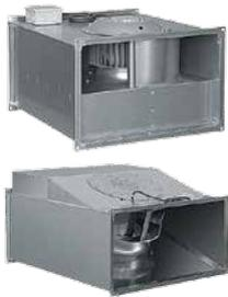
The fan housing and impeller are made of galvanised steel. The backward curved impeller (standard sizes from 40-20 to 90-50) or “free” impeller with blades bent backward (standard size 100-50). Single-phase and three-phase asynchronous electric motors are protected from overheating with the help of embedded heat contacts with remote circuit terminals. Operating resource is more than 40,000 hours.
