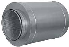
The silencer consists of two pipes of galvanized steel inserted one into the other. Sound absorbing material is a mineral fiber. Two modifications: 600 mm and 900 mm.
