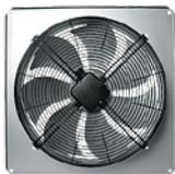
The fan housing and square wall-mounted panel are made of galvanized steel. The crescent blades are made of aluminum alloy and manufactured by Ziehl-Abegg AG, Germany. Single-phase and three-phase asynchronous electric motors are protected from overheating with the help of embedded heat contacts with remote circuit terminals.
