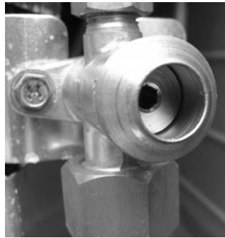
Fig. 6.10 Gas pipe Service valve (left figure) Liquid Service valve (right figure) <operate it with wrench> <operate it with hexagonal wrench> <the valve shown above is fully closed> <the valve shown above is closed>
