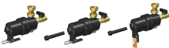
Closing the shut-off valve. Removing the magnet (turn it 90 clockwise). Opening the drain valve.
