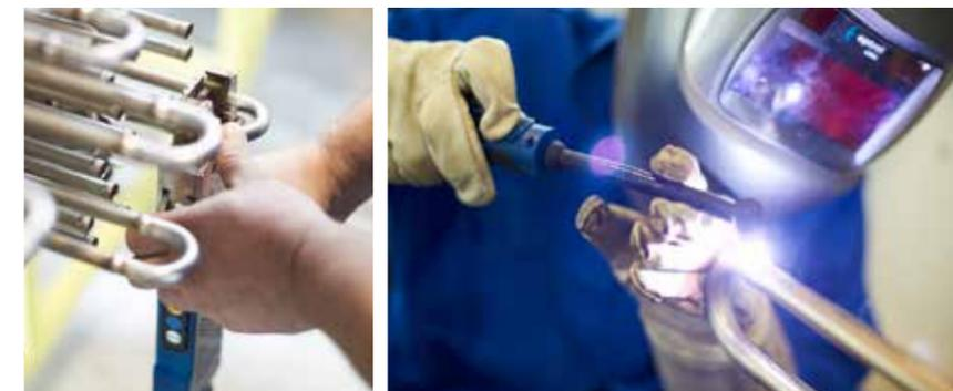
Modern technology also in detail: Orbital welding enables consistently high levels of seam quality for our products.
