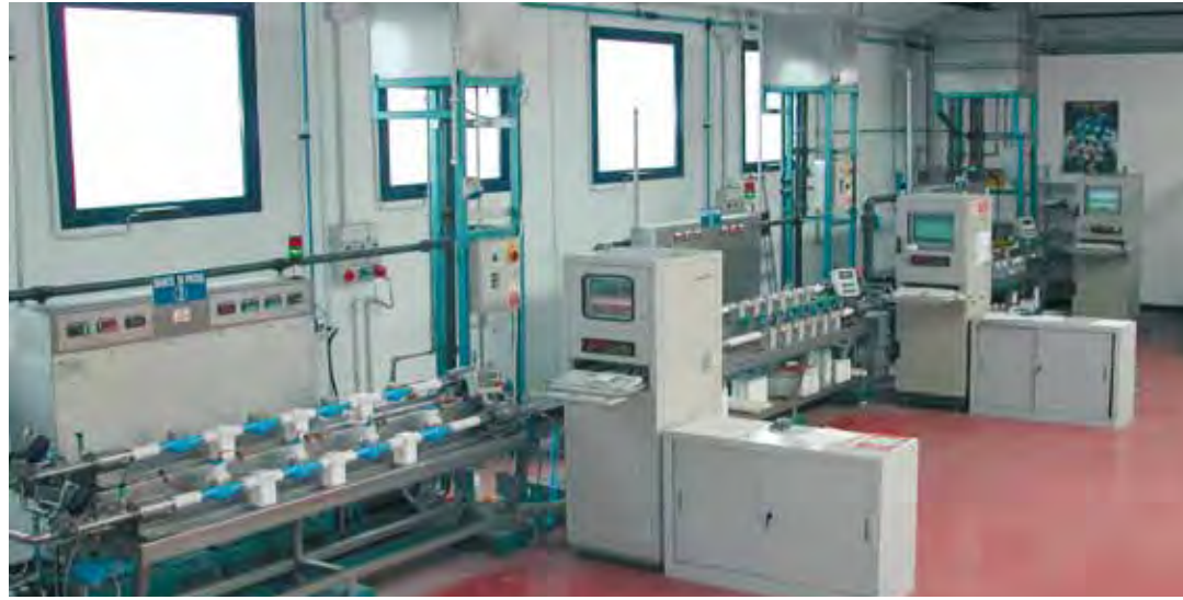
Banco prova per contatori domestici calibro da 1/2" a 2" Metrological test benches for water meters single and multi jet (from DN15 to DN50)
