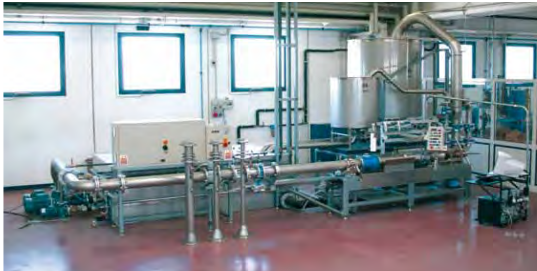
Banco prova per contatori industriali calibro da 2" a 8" Metrological test bench for waters meter woltmann type (from DN50 to DN200)
