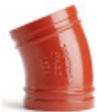
Series 230/16 Grooved elbow 22° DN50-200 20,6 bar (300 PSI) Ductile iron UL/ULC listed, FM approved
